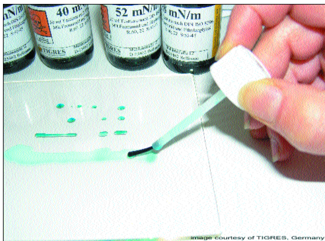
Evaluating substrate surface energy to indicate cleanliness.
